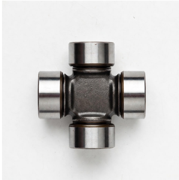
Figure 1: Picture of a typical u-joint that you can buy at any autoparts store. Shaft yoke ears connect to the 4 trunnions - one yoke horizontal and the other vertical
